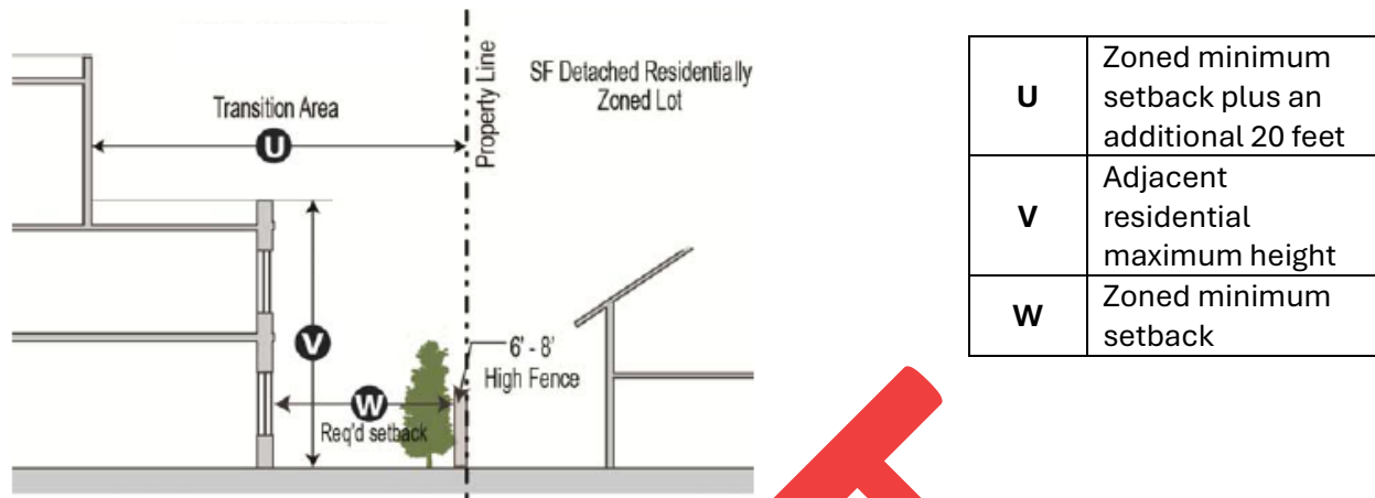
Figure 52-402C Illustration of Height Transition to Single-Family Detached zoned lot
